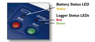
To **power down the logger manually**, press the green and red buttons simultaneously and hold them for 3 sec.
