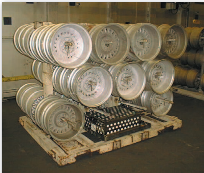
Furnace Tracker System for aluminium wheel heat treatment monitoring
